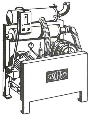
For intermittent use, in transferring material to VAC-U-MAX Hoppers in process machinery areas, a switch valve assembly is generally used in the vacuum line to the pump to return the hopper to atmosphere on the discharge cycle. Add to the system, a SVA-switch valve assembly, and the necessary length of plastic hose.
